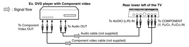
■ Selecting Component input mode Press INPUT SELECT repeatedly to select "COMPONENT" mode.
